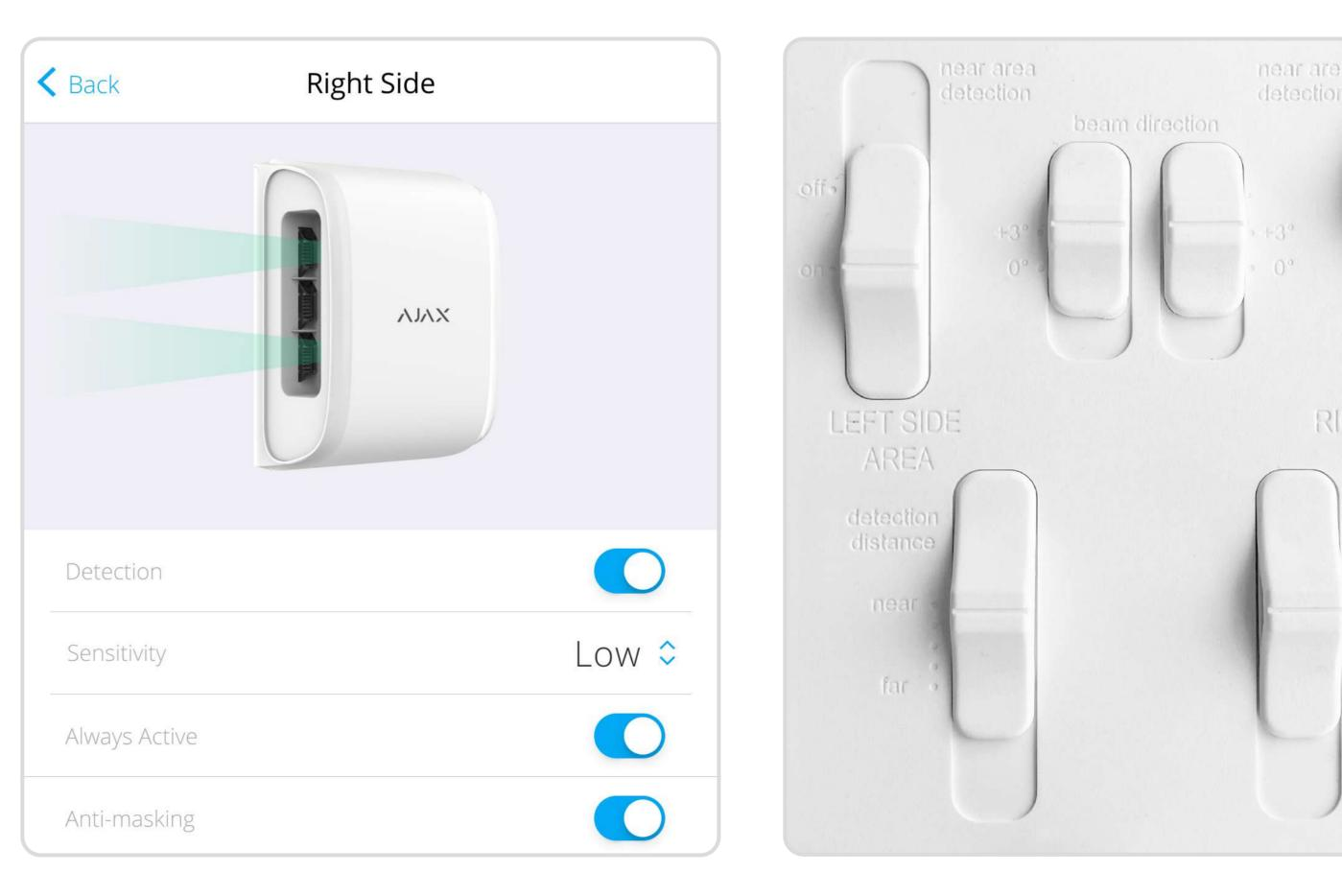
**Each side** of DualCurtain Outdoor has adjustable detection zone distance and direction. They help to adjust the detector according to the architecture and ensure accurate threat detection.
